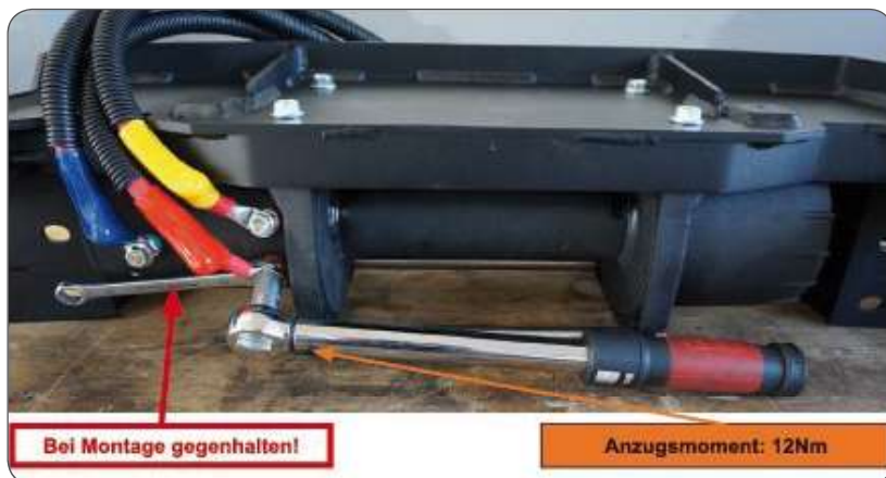
Abb. 12: Kabelmontage -Achtung: Symbolbild | cable mounting the image shows a symbolic picture
