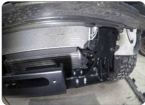
Abb. 05: Windenträger am Fahrzeug | winch carrier mounted to the car
