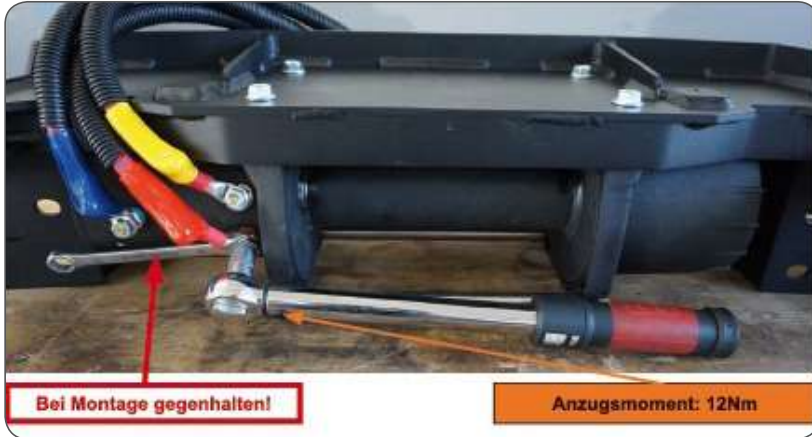
Abb. 08: Kabelmontage -Achtung: Symbolbild | cable mounting the image shows a symbolic picture
